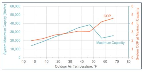
Figure 2. Illustration of ducted ASHP COP and capacity variance by outdoor air temp.
